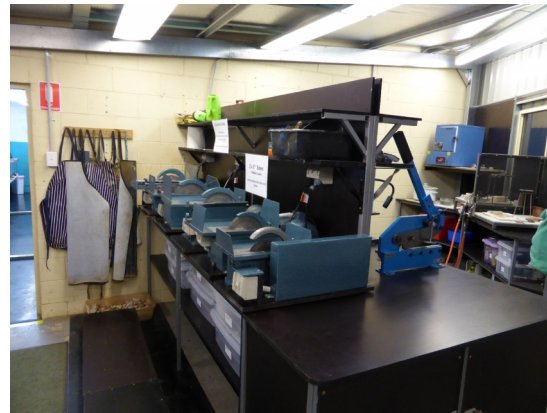
New Saw room area., we now have '5' diamond saws for hand use, separate areas for Tumbling, Dopping, marking out and tin oxide polishing. Plus adults and kids apron areas. (plus storage for BBQ and Laps)
